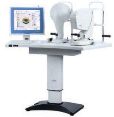
The two versions of the SCHWIND Combi Wavefront Analyzer integrate a range of unique functions and thus contribute to optimal surgical and diagnostic decision-making.
