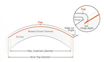
Particularly in the excimer laser treatment of hyperopia and mixed astigmatism, the SCHWIND ATOS can be used to create flaps of various diameters. This precision technology from SCHWIND is based on a sophisticated contact glass design and can be used highly flexibly, even for large flaps and treatment diameters.
